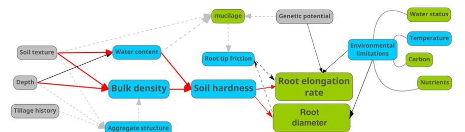
Conceptual diagram of factors affecting root growth rate in *OpenSimRoot*. Red arrows are links newly implemented in this study; dashed lines are planned but not yet implemented.
