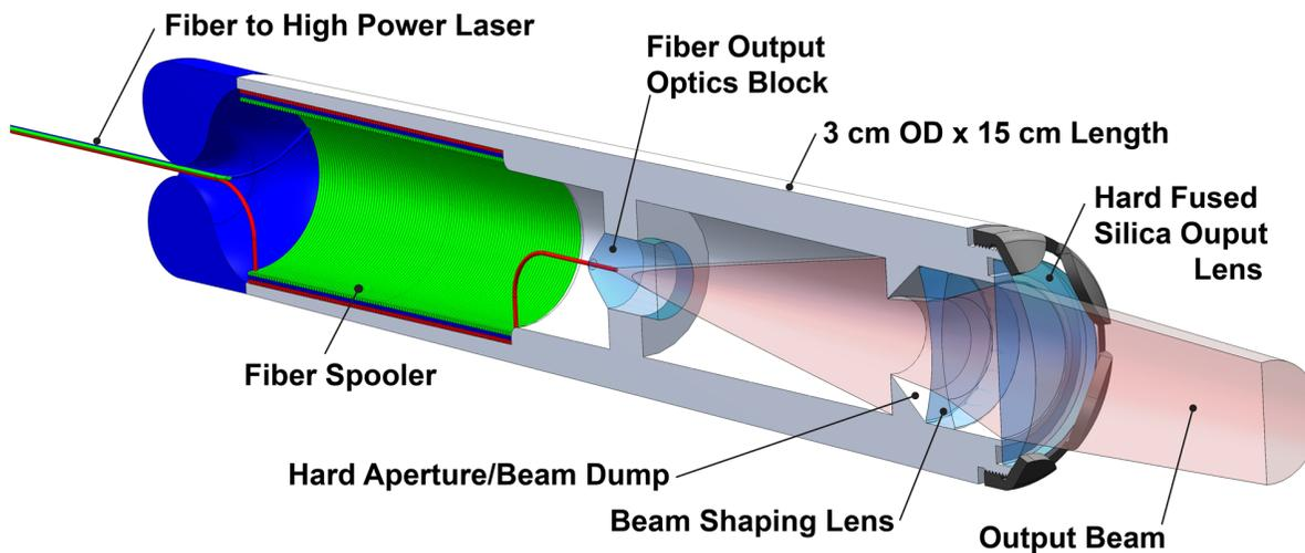
The fiber optic line can be wound quite tightly, meaning that 100+ meters of fiber can be accommodated onboard the penetrator, giving the probe a significant range.
