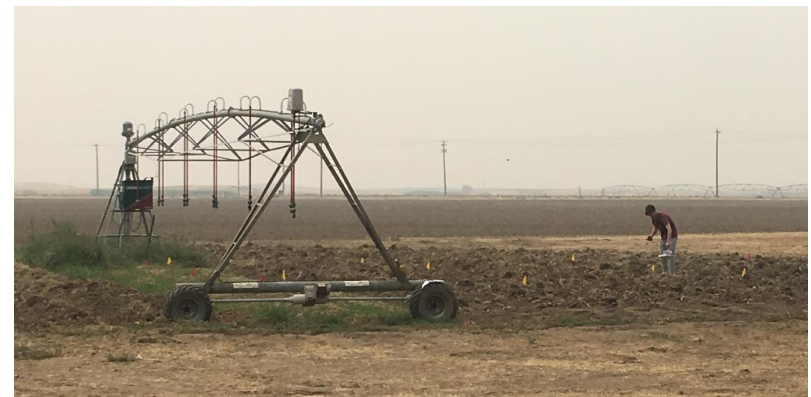
Collecting data from tags buried under a 10m radius center pivot irrigator. There were 18 total tags buried in this field.
