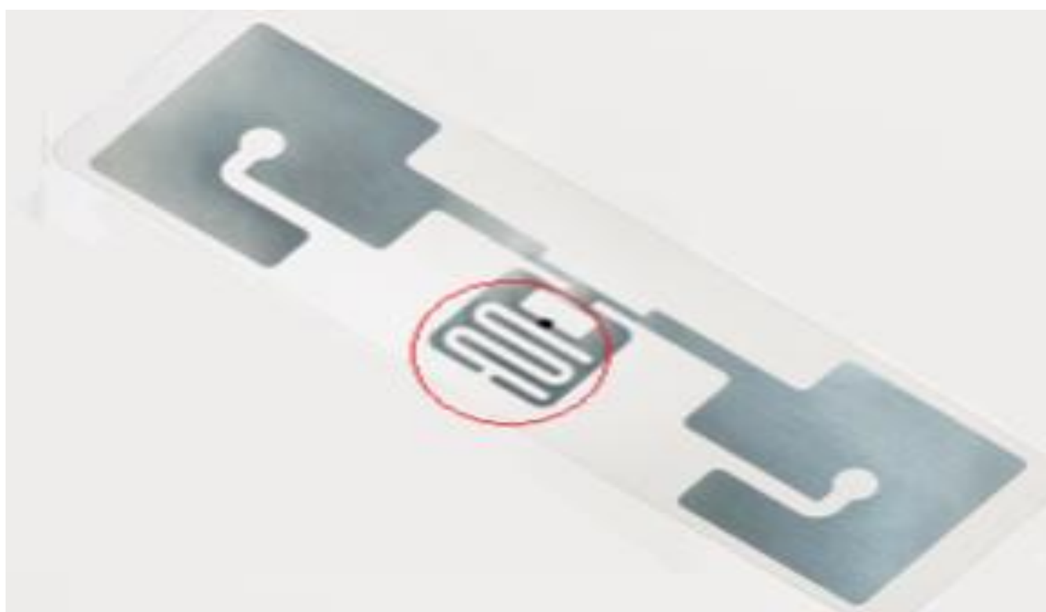
Close up of SmarTrac's Dogbone RFID tag with the moisture sensitive area circled in red.
