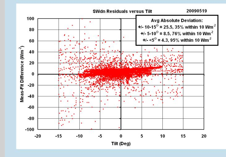
Long et al. (2010) show that the tilt correction methodology corrected 90% of the data to within 10 Wm<sup>-2</sup> for tilt of +/- 10° or less, with an average absolute deviation of 5.2 Wm<sup>-2</sup>, and 95% if the data within 10 Wm<sup>-2</sup> for tilt of +/- 5° or less.
