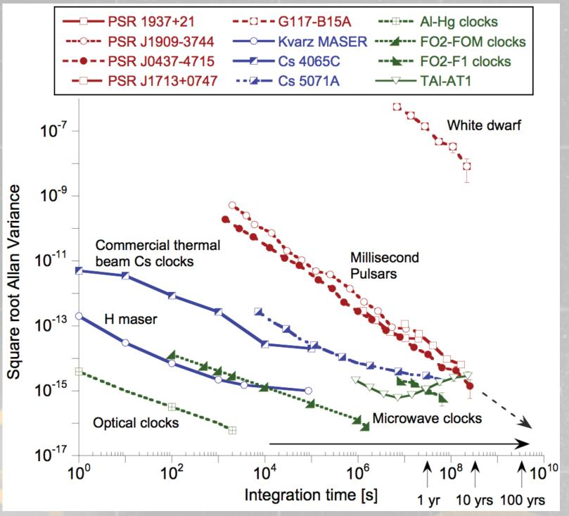
**Figure 1** - Comparison of terrestrial and astrophysical clocks. The frequency stability is expressed in terms of square root Allan variance (y-axis), and the x-axis represents the integration time. Optical clocks are currently the best ones, but the long-term trend of the best millisecond pulsar (dashed arrow) shows that MSPs may compete if we allow a long integration time. See (Hartnett and Luiten 2011) for details.
