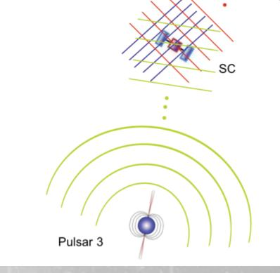
**Figure 2** - A three dimensional position fix can be obtained by observing at least three pulsars. Given three well chosen pulsars, there is only one unique set of pulses that solves the location of the spacecraft (SC). Figure adapted from (Sheikh 2005, 200).
