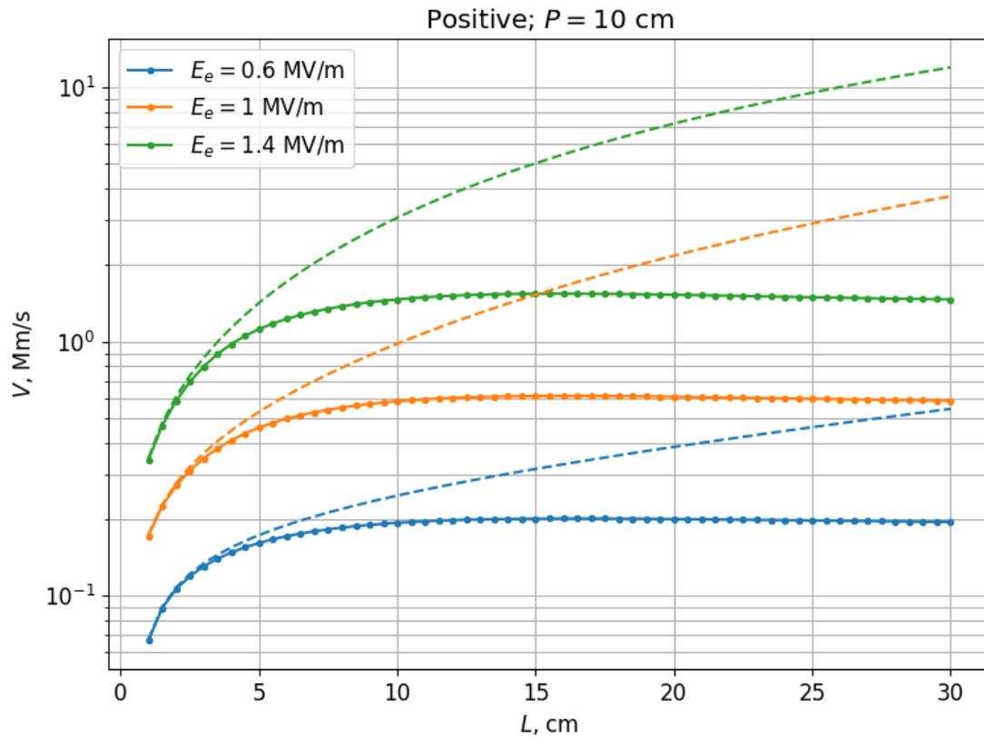
Here, the dashed lines are for isolated streamers. The reason for the observed stabilization is that the external field  $E_e$  does not penetrate beyond distance  $\sim P$  behind the streamer tips, so the effective length of the streamer remains to be of the order of  $P$  (or  $P/2$ ).
