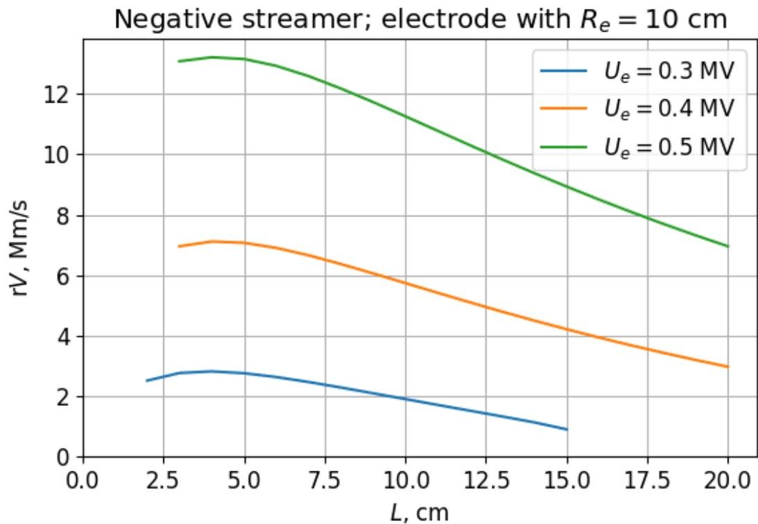
In the negative streamer case, the streamer stops because the field falls below the propagation threshold.
