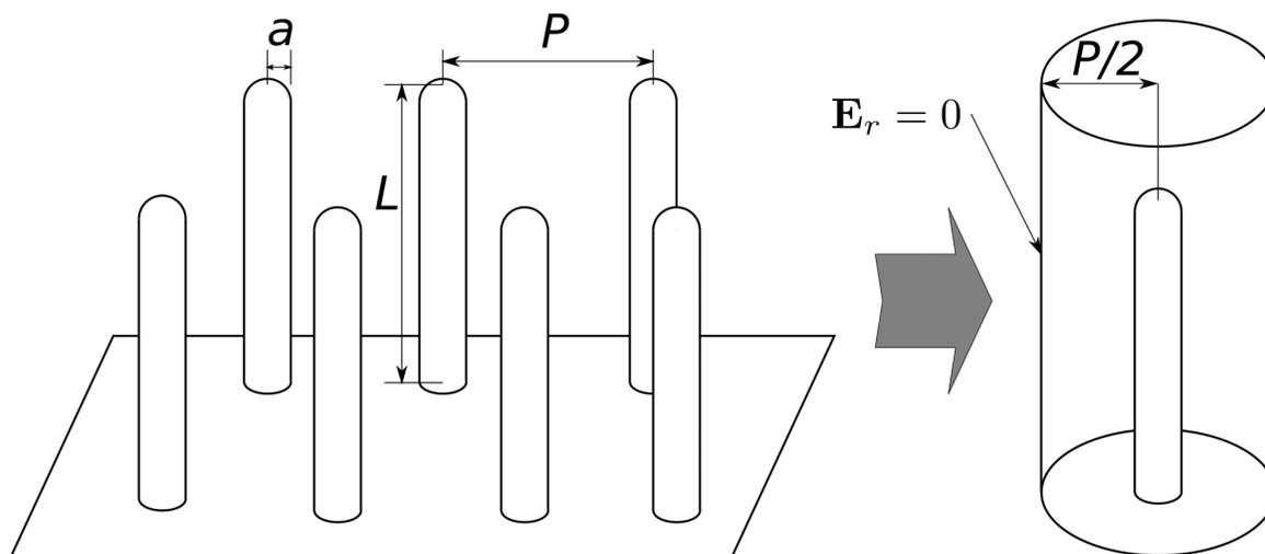
Because the effect of the cylinder walls is to limit the field at the tip  $E_m$ , the resulting effect on streamer parameters is stabilization of velocity and radius as  $L$  grows above  $P$ :
