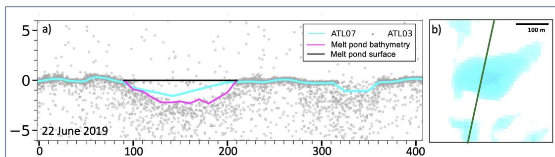
**Figure 4.** Melt pond detection on sea ice in the Lincoln Sea (adapted from Farrell et al., 2020, see Figure 2a MP 9). (a) ATL03 photon heights (gray), ATL07 height (cyan), and UMD-MPA-derived melt pond surface (black) and bottom (magenta) elevations. (b) Validation of melt pond in Sentinel-2 imagery captured 37 minutes prior to the ICESat-2 pass (RGT 13070304).
