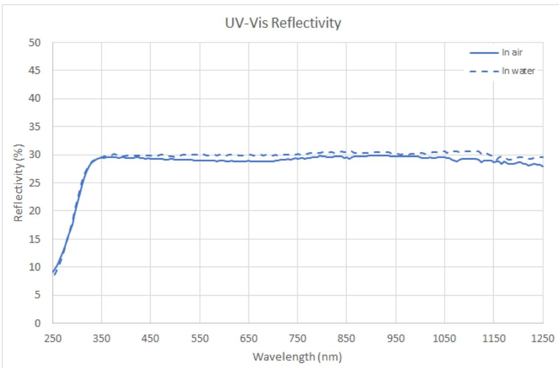
Figure 3: UV-Vis Reflectivity of 0.5mm thick layer of 25P45 material. Reflectivity was measured as in (Chamberlin, 2020).
