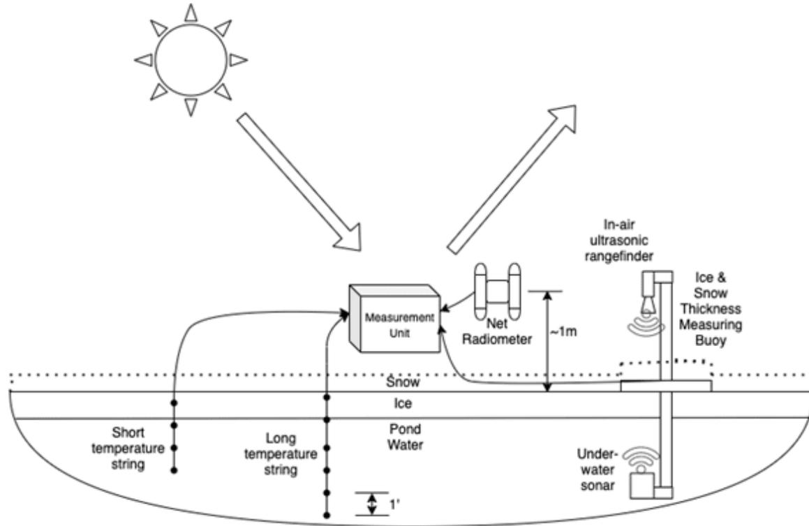
Figure 1: Side view schematic of measurement systems.
