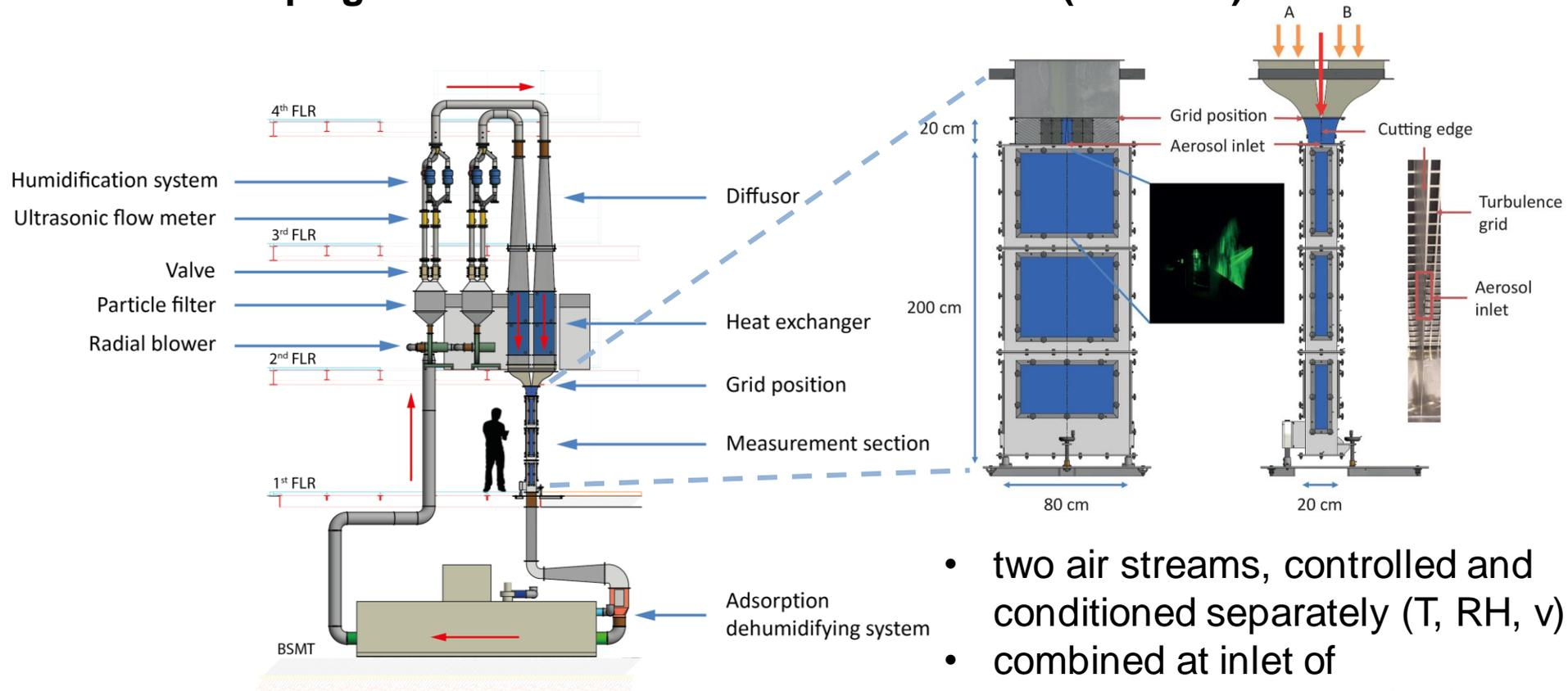
turbulent moist-air wind tunnel LACIS-T
