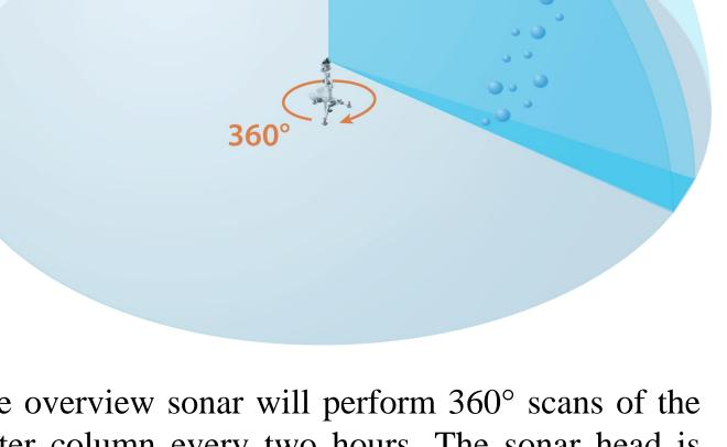
The overview sonar will perform 360° scans of the water column every two hours. The sonar head is mounted so as to orientate the swath vertically. All gas bubbles present within a 150 m-radius hemisphere centred on the sonar will be detected.
