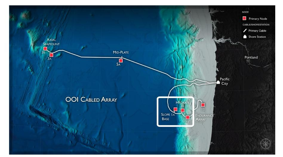
2015, Since the Ocean Initiative's Observatories (OOI)Cabled Array observatory provides power two-way communication to the SHR. making it an ideal site for continuous long-term monitoring work.
