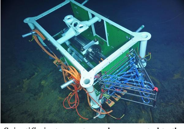
Scientific instruments can be connected to the OOI network via subsea junction boxes. (Credit: University of Washington/NSF Ocean Observatories Initiative).
