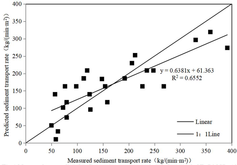
**Fig.4 Measured vs. predicted sediment transport rate (using the model:  $ST=76.857+ 13.346S-228.027 C$ )**
