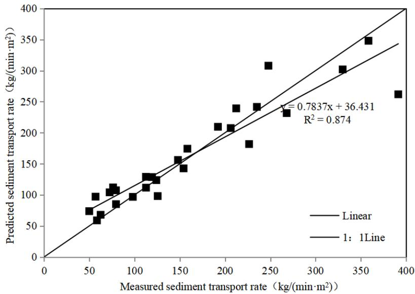
**Fig.5 Measured vs. predicted sediment transport rate (using the model:  $ST=45.571e^{0.485I+0.075S-1.423C}$ )**
