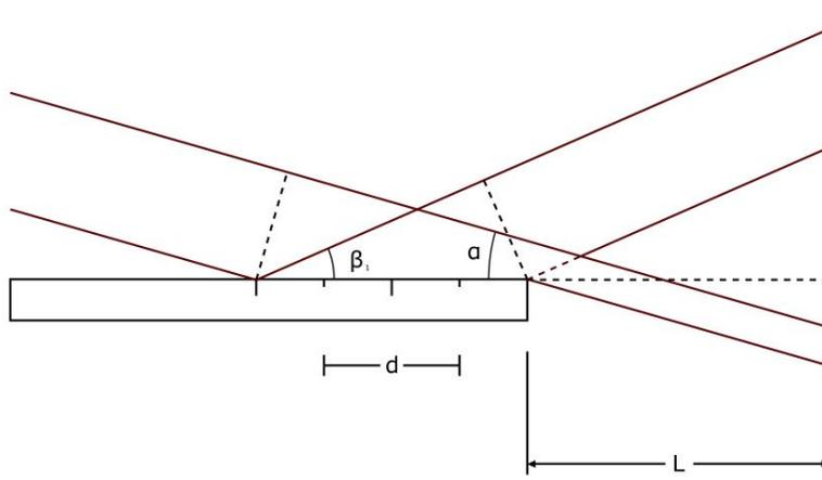
Figure 2: Path length from the angles of reflection
