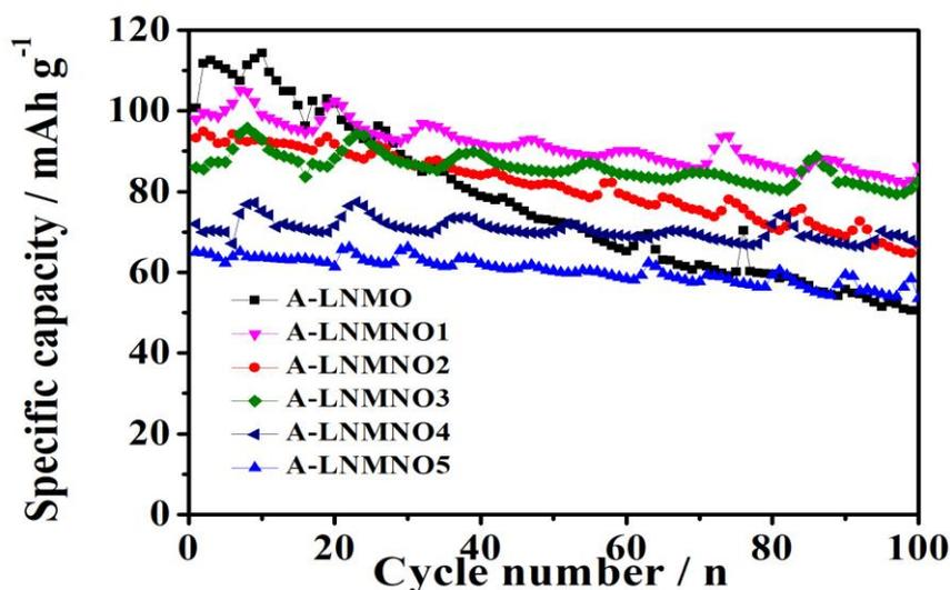
Fig. 8. Cyclic performance of LNMOs at room temperature
