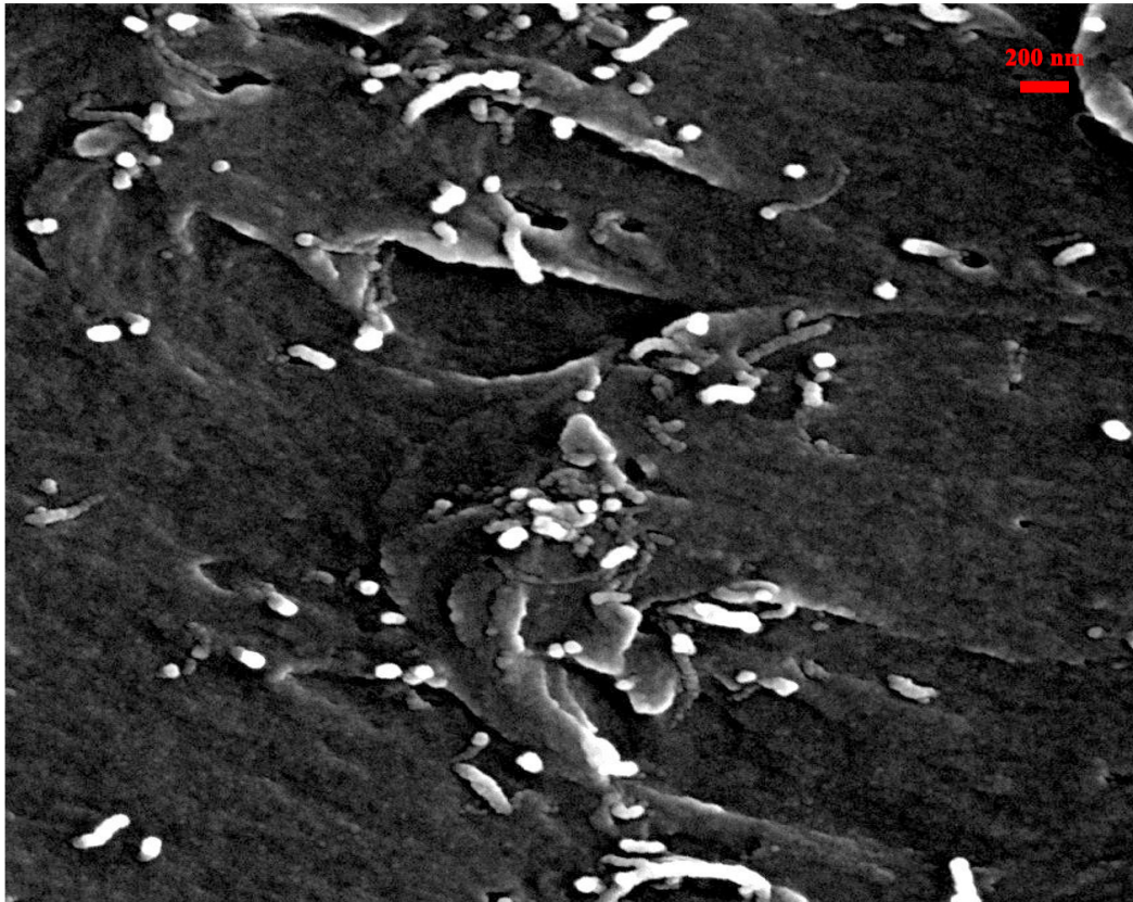
Figure 6. Scanning electron micrographs of the epoxy matrix composite materials reinforced with multi-walled carbon nanotubes.
