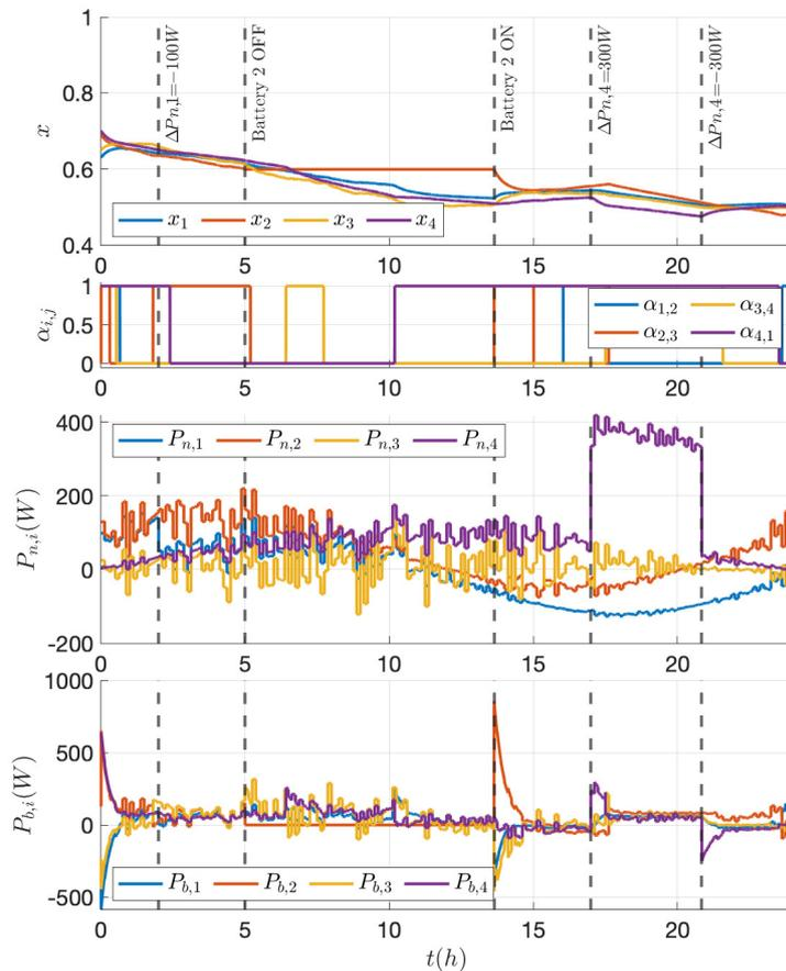
**Figure 6** For  $\varepsilon = 0.005$  and  $\varepsilon_M = 0.03$ , we have from the top to the bottom: the  $x_i$ ,  $\alpha_{i,j}$ ,  $P_{n,i}$  and  $P_{b,i}$  evolutions, respectively. There are unintentional connection/disconnection of any element of the MGs marked by the discontinuous lines.
