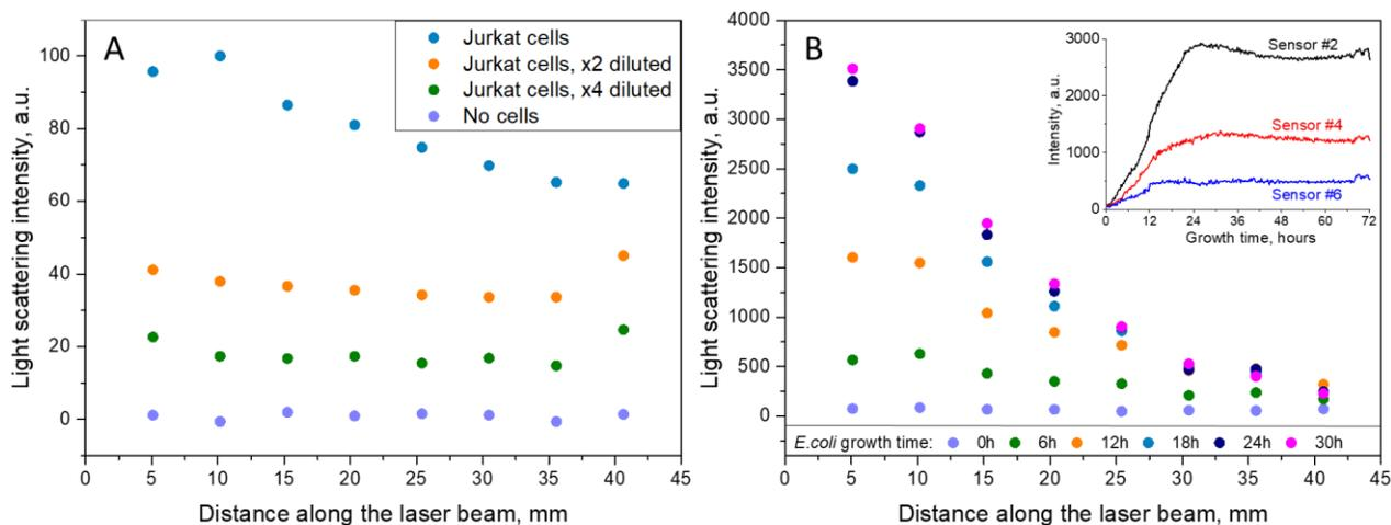
Figure 3. Testing of the prototype with cell cultures. A: Jurkat cells give low but detectable signal, but the attenuation of laser beam is visible only for maximal concentration ( $\sim 10^6$  ml $^{-1}$ ). B: Continuous monitoring of the *e.coli* bacteria growth.
