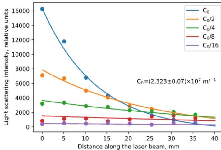
Figure 2. Experimental measurements (points) and theory (lines) for polystyrene beads in different concentrations. The first concentration  $C_0$  and the proportionality coefficient are determined by fitting.
