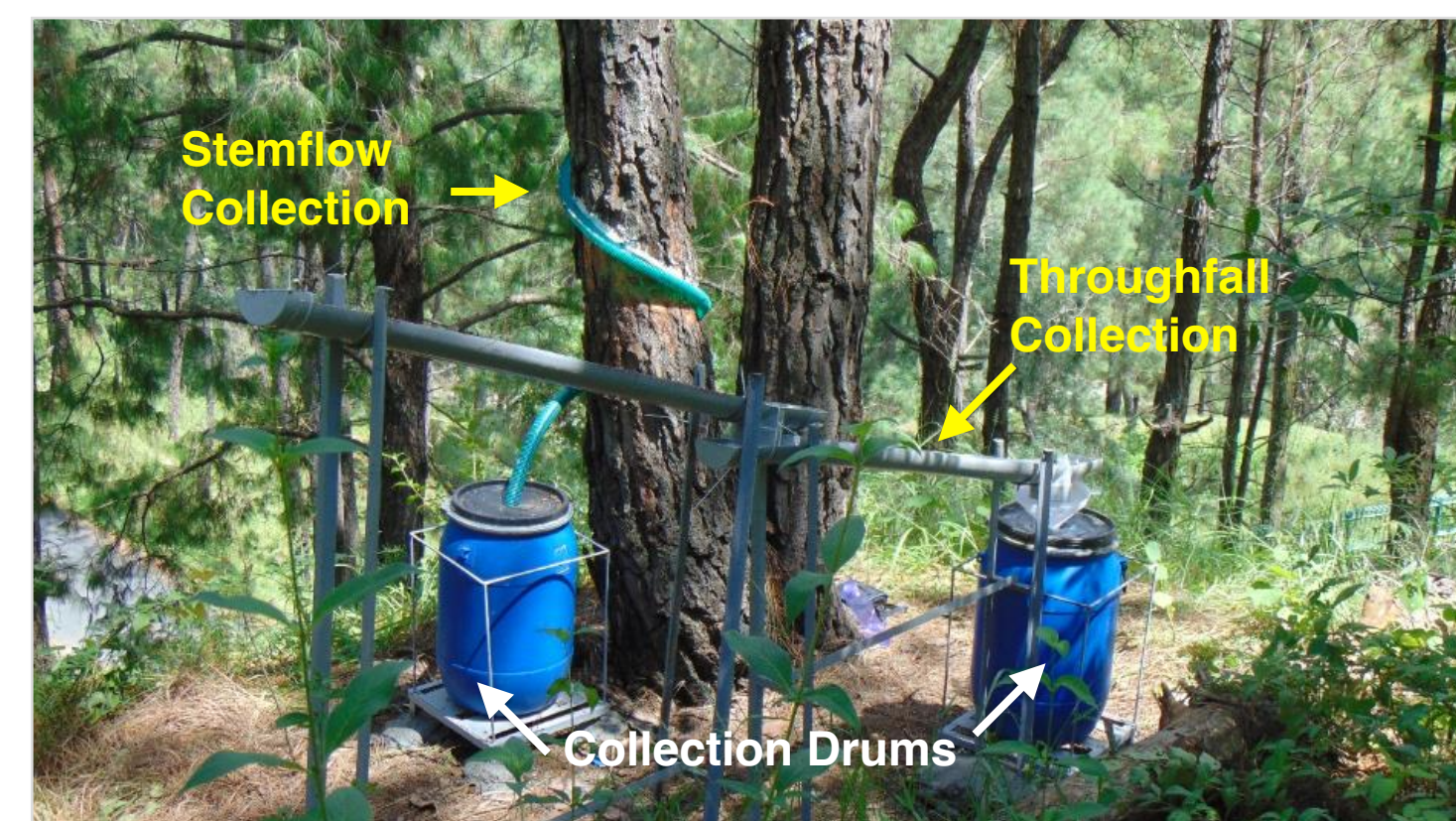
Existing Setup at Hydrological Study Field at Almora, Uttarakhand, India
